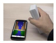
**Figure 2.** An ordinary whiteboard wiper was used as a magnetic joystick.
